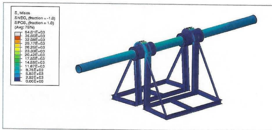
Figure 35: FE Results Case 2 – Stresses.
