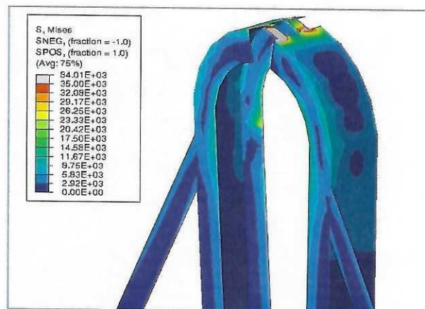
Figure 36: FE Results Case 2 – Yoke to Pipe Clamp.
